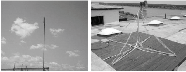
Figure 1: VLF receiver systems at Belgrade station: AbsPAL (left) and AWESOME (right) antennas.
