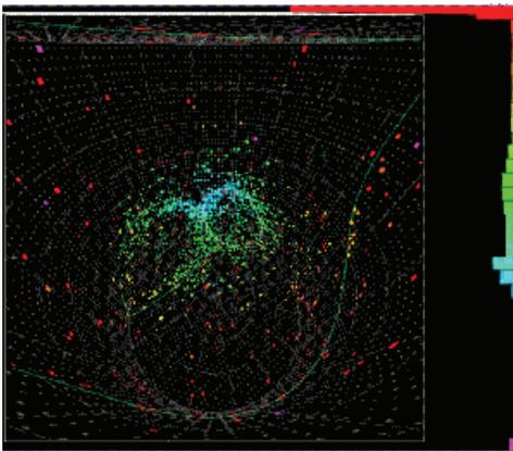
The first T2K event seen in Super-Kamiokande. Each dot is a photo multiplier tube which has detected light. The two circles of hits indicate that a neutrino has probably produced a particle called a  $\pi^0$ , perfectly in time with the arrival of a pulse of neutrinos from J-PARC. Another faint circle surrounds the viewpoint of this image, showing a third particle was created by the neutrino.
