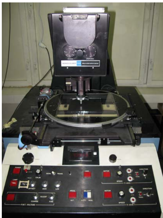
Figure 3. The Perkin-Elmer historic microdensitometer of LAPD in Sofia - PDS 1010 plus still used for some tests and plates scan calibration.
