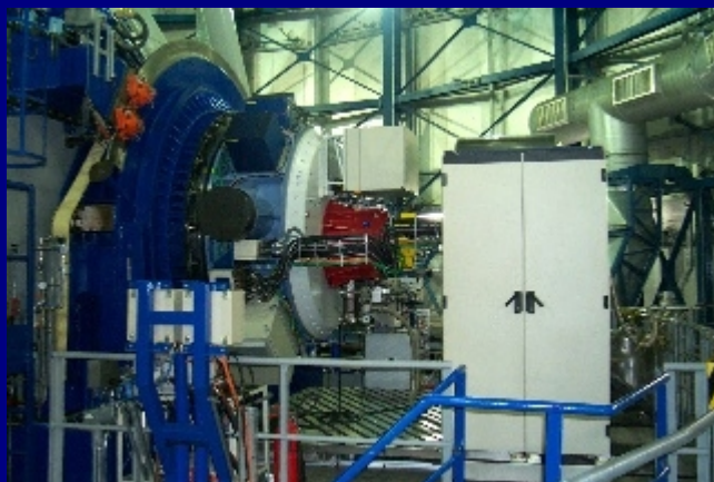
NACO mounted on UT4 1-5 micron imaging polarimetry Wollaston prism
