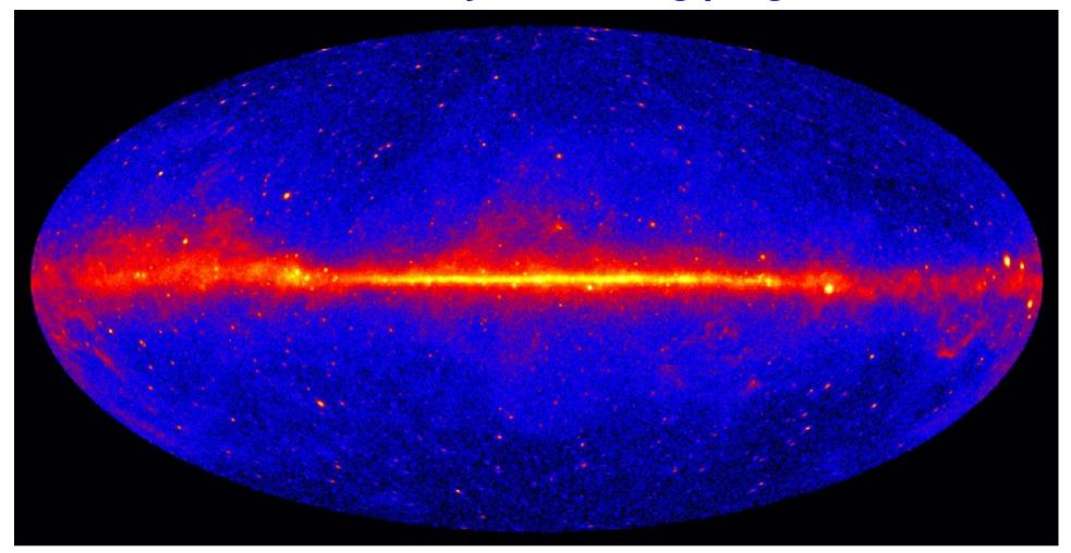
A view of the entire sky at energies between **1GeV** and **300GeV**, obtained after **two years** of regular monitoring with the Fermi/LAT. Thanks to its orbit and large field of view, the instrument performs an **entire sky scan every 3hr**. The observations are built up to produce an increasing sensitivity detection map. We note both **diffuse emission** and **point sources**.
